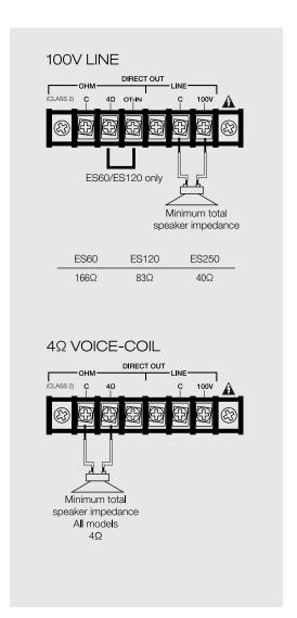
NOTE: Only connect one output – either 100V or  $4\Omega$
