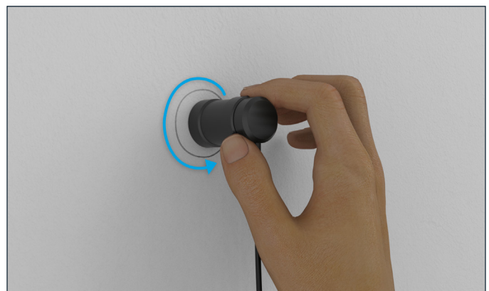
Figure 5: Slowly circling probe around marked disc location
