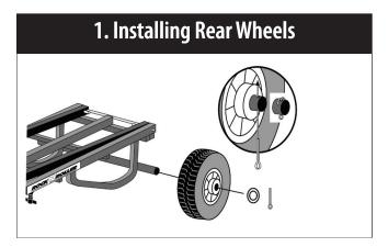
Gently slide wheel over axle as shown. Do not force wheels onto axle. It is recommended to lubricate axles with light grease before installing. Install cotter pins and bend ends outward.
