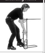
Loosen wingbolts 1/4 turn. Step on rear axle and push in extension stop button. Pull up on frame as shown until stop button engages. Retighten wingbolts.
